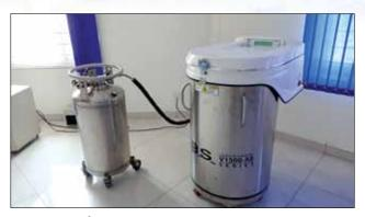
Fig. 62. Liquid Nitrogen Vapour Storage System
